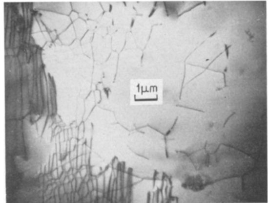
Figure 9 Networks in the (111) plane. Crystal deformed 5% at 720°C under a stress of 280 kg/cm 2 . \langle 110 \rangle approximately along the direction of the marker.
